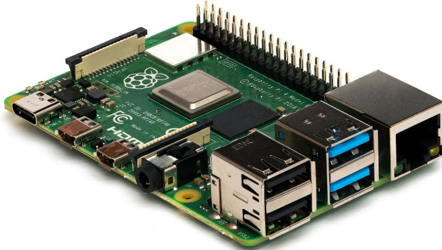
Figure 7 – Raspberry Pi single board mini-computer
