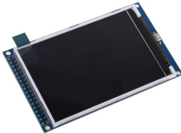
Figure 8 – 3.5" 320x480 pixels display module based on the ILI9481 controller
